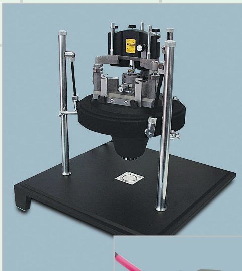
Solver P47H with AFAM set up
